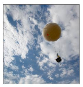
Meteorologists attach equipment to large helium filled balloons to monitor temperature, air pressure, humidity, wind speed and direction and cosmic rays in the atmosphere. Because helium is lighter than air, the balloon rises high into the atmosphere where the readings can be taken.
