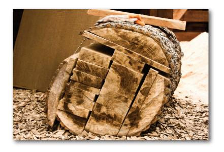
Wood comes from trees. Logs are cut from tree trunks and sawed into planks that can be used for a variety of building purposes.
