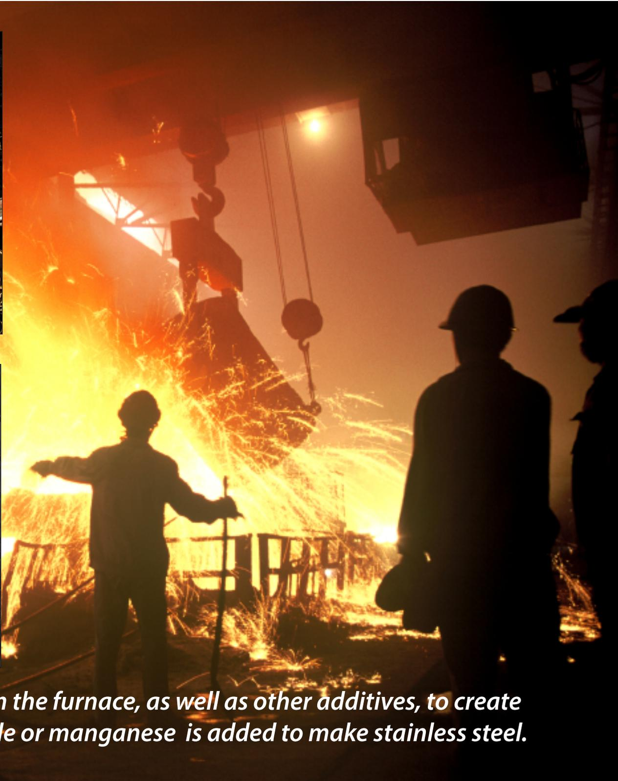
*Scrap metal is added to the molten iron in the furnace, as well as other additives, to create different types of steel. For example, nickel or manganese is added to make stainless steel.*
