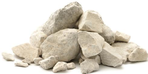
*Flux materials*, such as limestone or dolomite, are added to the molten iron. The limestone combines with the impurities in the molten iron, making them easier to remove.
