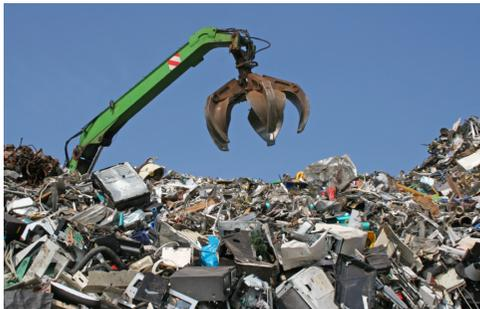
*Scrap steel* is added to molten iron. The scrap steel includes off-cuts from the steel making process as well as recycled steel that comes from household collections and scrap metal yards.
