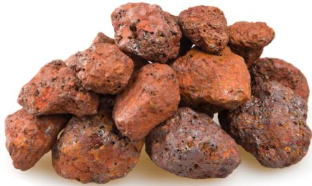
*Raw iron ore* is crushed and magnetic rollers extract the fine grained iron from the rock dust. This is then heated to make the particles stick together, forming small rocks. This process is called *sintering*
